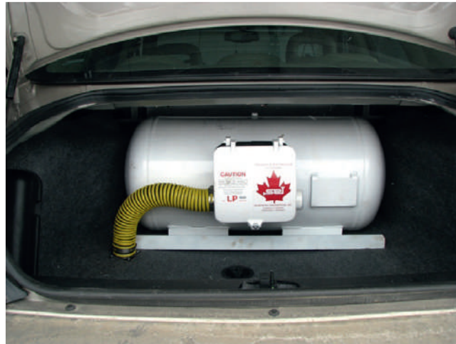
Figure 2.310 Propane tank. (Source: http://www.rasoenterprises.com )
